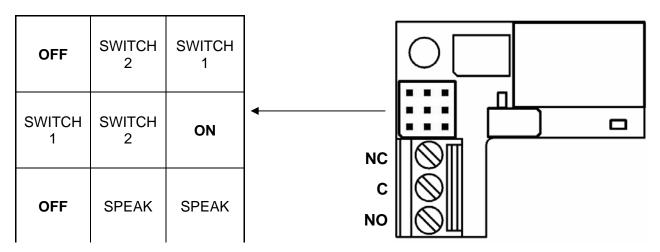
The switch input is available both normally open (between clip **C** and **NO**) as well as normally closed contact (between clip **C** and **NC**).
